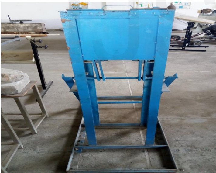
Figure 6: Front View of Fully Fabricated Fly Ash Brick Machine.
