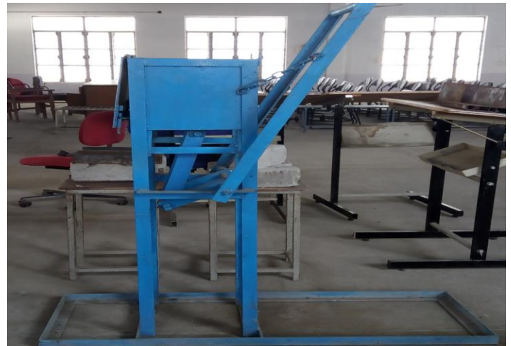
Figure 8: Side View of Fully Fabricated Fly Ash Brick Machine.
