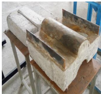
(c) Isometric view ohm shape brick die
